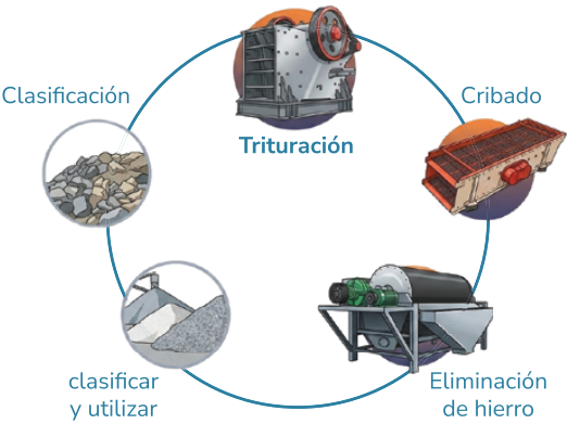
Figura 3.31. Reciclaje del material estéril Fuente: Tomado de: Jordan (2021). How to make recycled concrete aggregate: Process and uses. https://www.ftmmachinery.com/blog/how-to-make-recycled-concrete-aggregate-and-what-is-it-used-for.html
