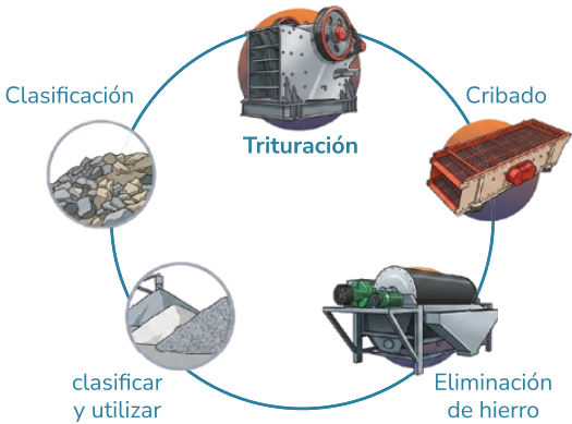
Figura 3.30. Reciclaje del material estéril Fuente: Tomado de: Jordan (2021). How to make recycled concrete aggregate: Process and uses. https://www.ftmmachinery.com/blog/how-to-make-recycled-concrete-aggregate-and-what-is-it-used-for.html
